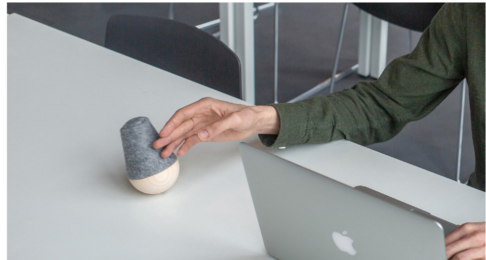
Figure 5. Topplr, a peripheral music controller, allowing users to skip songs by tumbling it down (example of input-only interface)
